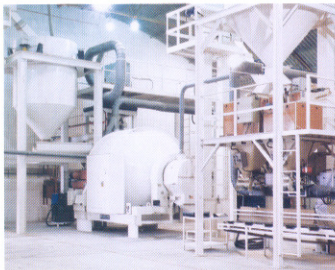
The hopper (at left) feeds clay or quartz into the 700-TSC-180 rotary mixer. Chemicals are sprayed as the batch rotates.
