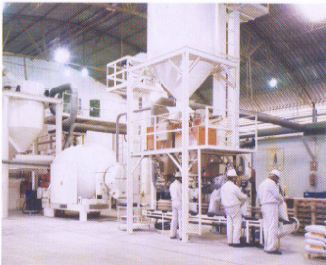
Workers package insecticide after it has been mixed by the rotary mixer (left).
